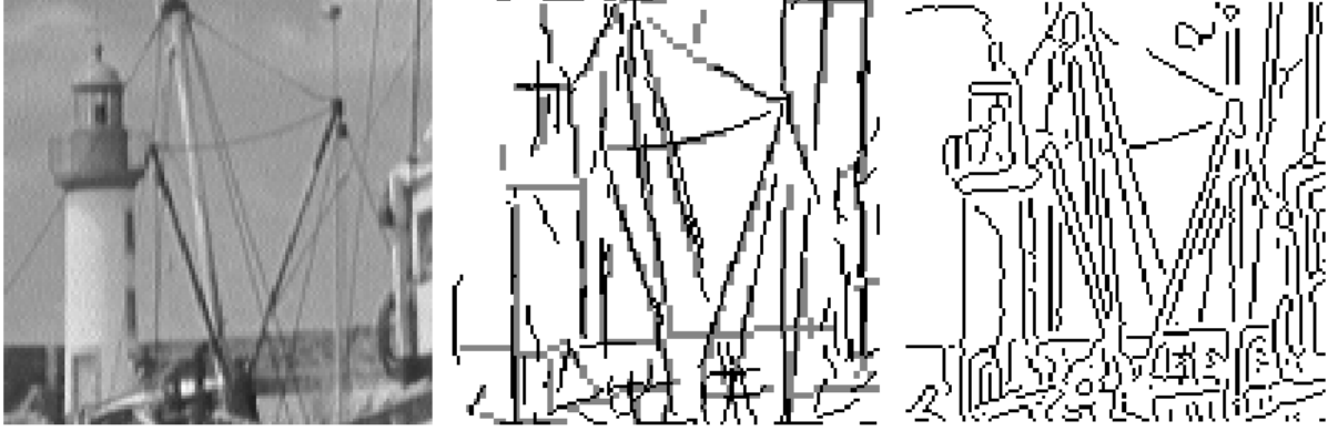
Figure 22: Edge extraction using the multi-scale representation. (Left) 128 \times 128 pixel image "Boats". (Middle) Edges extracted by sparse Gabor wavelets. 1st scale and 2nd scale edges appear in black. The 3rd scale edges appear in gray, they are plotted larger since the 3rd scale is downsampled and offers coarser spatial localization. (Right) Edges extracted by Canny method [Canny, 1986; Deriche, 1987]. The SEC method extracts edges which are subjectively more accurate. Reconstruction of the image using these edges revealed qualitatively better results (see [Fischer et al., 2007a]).
