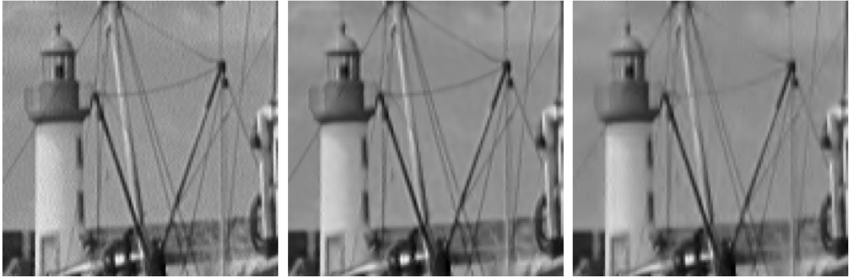
Figure 23: Denoising results. ( Left ) This 120 \times 120 detail of the image "Boats" is corrupted by Gaussian noise for a Peak-Signal to Noise Ratio (PSNR) of 20.22 dB and contains an important level of noise. ( Middle ) After denoising by bi-orthogonal wavelets 'db4' and soft-thresholding a high level of artifacts appears, PSNR=24.65 dB. In "Boats" many details, i.e. the wires, appear smoothed and almost disappear while some noise points still remain. ( Right ) The image denoised by sparse log-Gabor wavelets shows a dramatic decrease of the level of artifacts, moreover some important details now appear preserved and the blur is lower. The PSNR shows an important improvement up to 25.30 dB.
