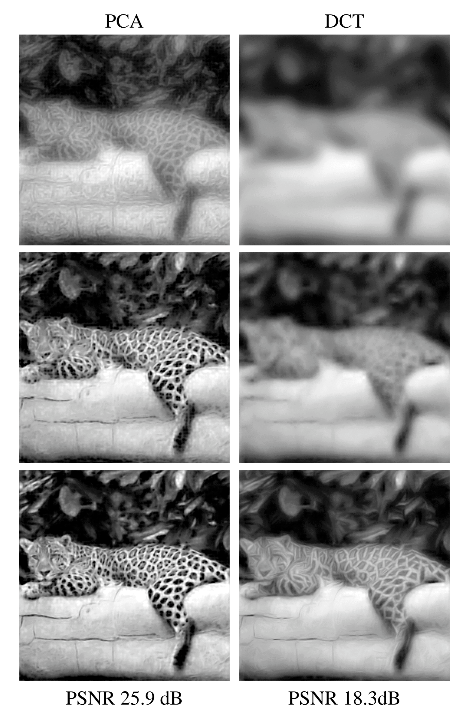
FIGURE 5. Warplet reconstruction results. Coding and synthesis using the warplet domain using mean only, mean plus 3 modes and mean plus 15 modes on jaguar image. Comparisons with DCT coding of warplet domain using equivalent number of coefficients.
